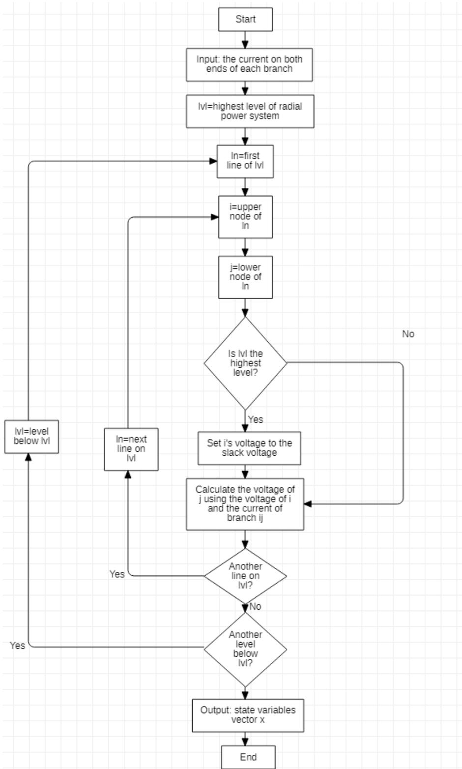
Figure 9: Forward Sweep Flowchart
